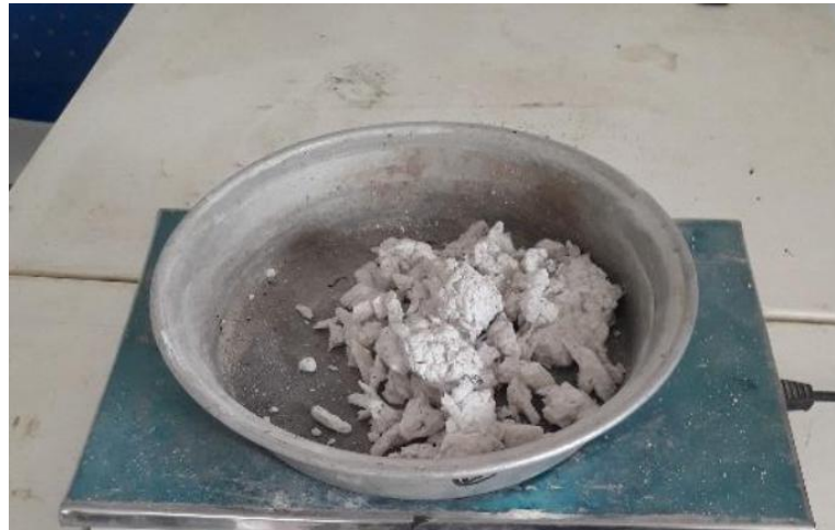
Figure 5: Marble exhibits a plastic (paste-like) consistency after water absorption
