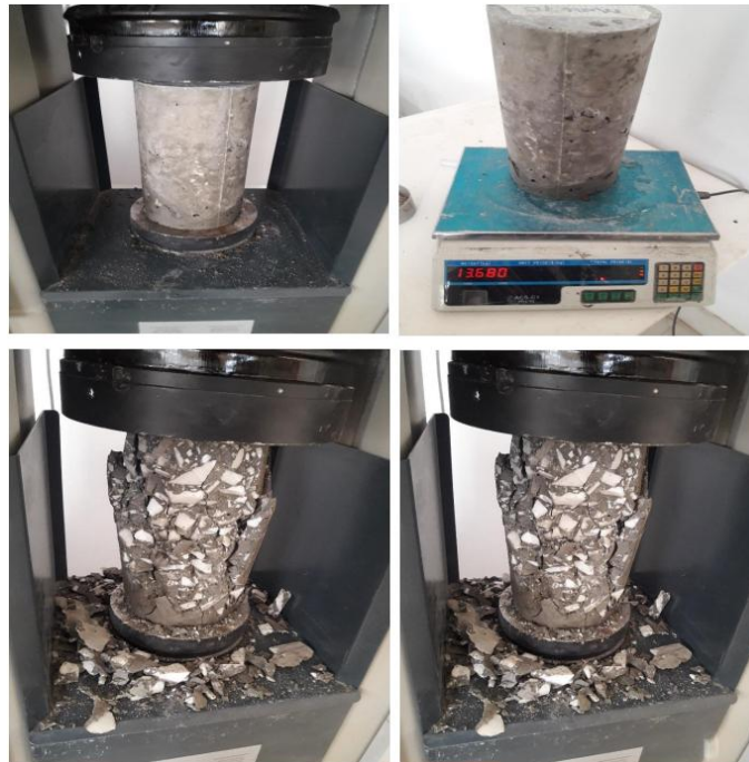
Figure 7: Marble concrete cylinders under compressive machine
