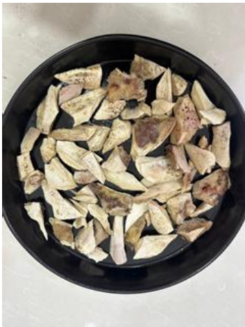
(a) removal organic bone and whitening by heat treatment
