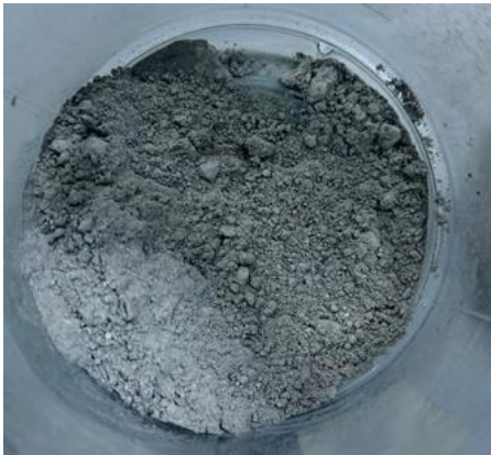
(f) heating the powder to 650°C
